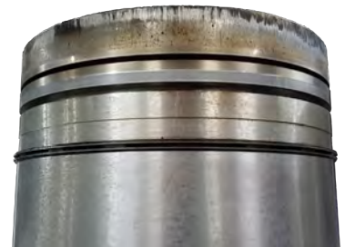
A VHP Series Five piston after field validation illustrates reduced carbon deposits
