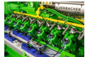
HanseWerk Natur, an E.ON company, is showcasing a flagship CHP project in Hamburg. The 1 MW Jenbacher J416 is optimized for pipeline gas operation and high total efficiency. Additionally, the engine can run on a variable hydrogen mixture from 0% up to 100% (100% H<sub>2</sub> for short-term demo operation). This is powerful proof that our Jenbacher Type 4 engines can operate exclusively on hydrogen and demonstrates the convertibility of existing engines to 100% H<sub>2</sub> operation.
