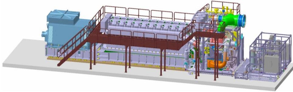
**Engine module separated in generator, engine, TCM and Aux Modules**
